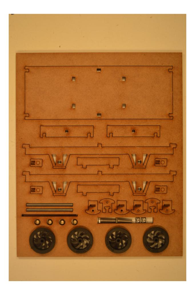
Locate the 2 sole bars and the 4 brass bearings.Press the bearings into the holes in the sole bars ensuring the etched lines on the sole bars are to the outside and the bearing flanges are to the inside.
