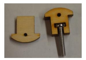
Finally fit the buffers and make up the coupling hooks using the supplied rod.
